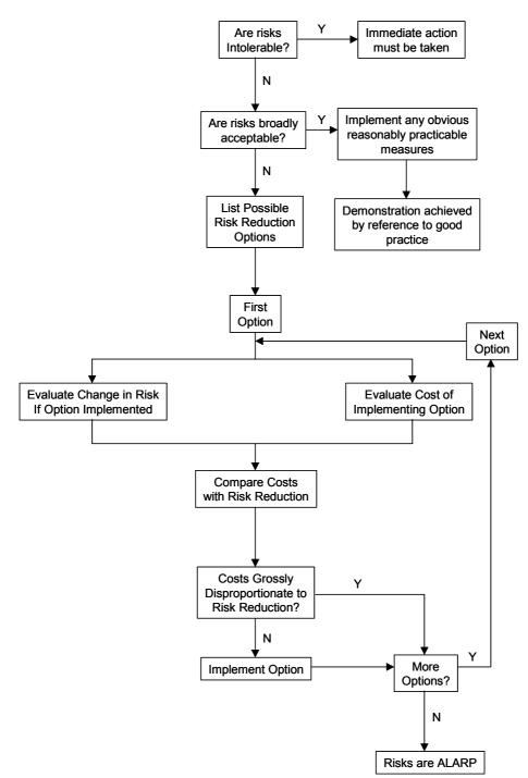
Figure 8.2 ALARP Determination Process
