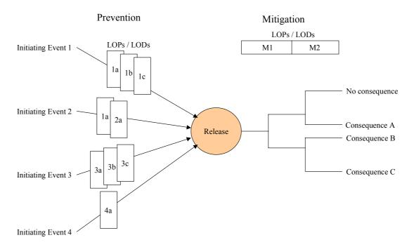
Diagrams such as that shown in Figure 1.2 are known as 'bow-ties'. With reference to the diagram, there are several important points to note:
